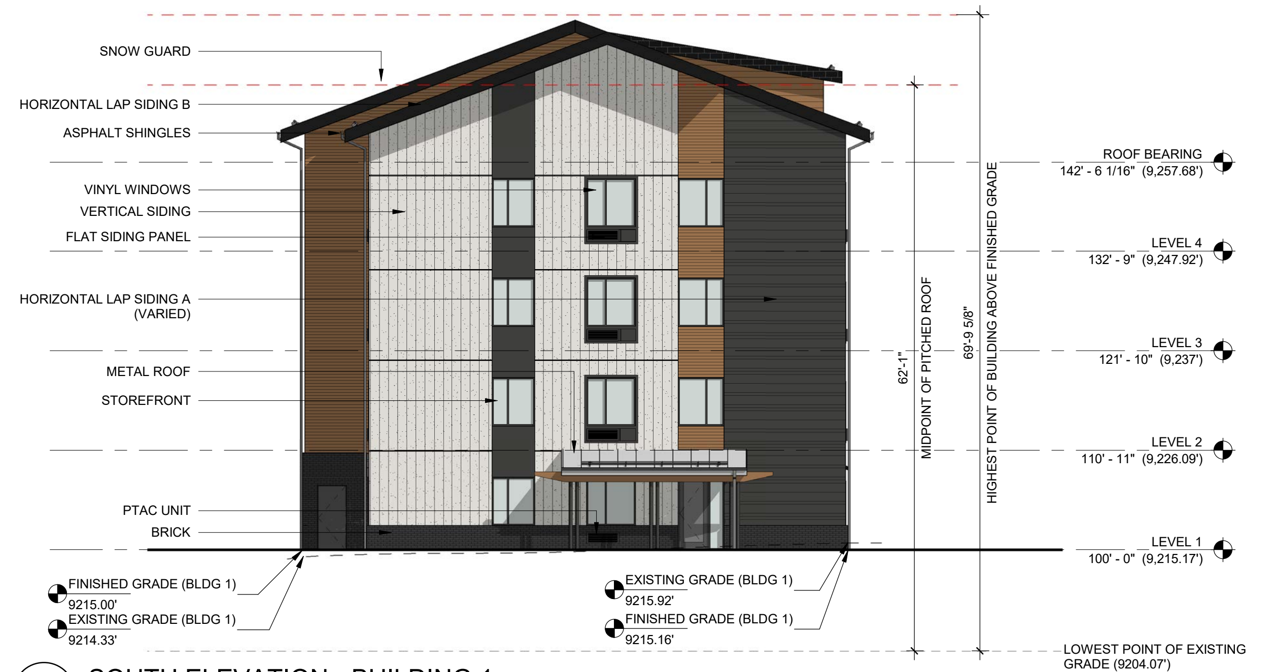
SOUTH ELEVATION - BUILDING 1 3/32" = 1'-0"
